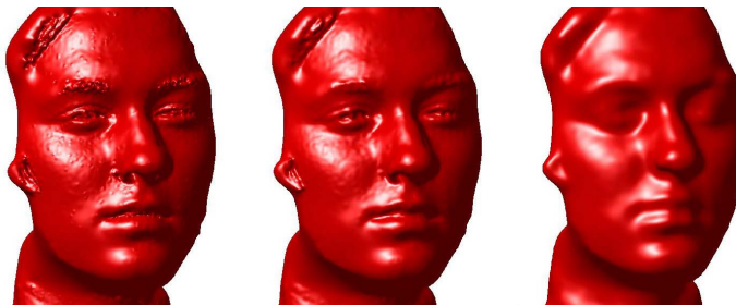
Figure 3.8: A head model reconstruction with different regularization parameters. The left image uses the parameters chosen by the automatic validation procedure proposed in Section 3.8, which leads to accurate results. For some applications, a smoother surface (centre) may be preferable. Additional smoothing without re-fitting can be obtained by just excluding the finest scales during evaluation as demonstrated in the right figure.
