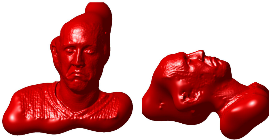
Figure 3.15: The head reconstructed with the parameters chosen by the validation process and \sigma_0 = 0.5 in units of the object diameter.
