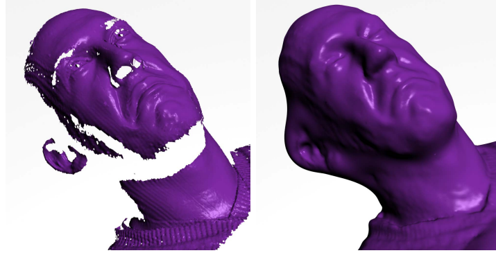
Figure 3.10: Holes due to occlusions in the scanning process (left) are filled by the implicit surface (right).
