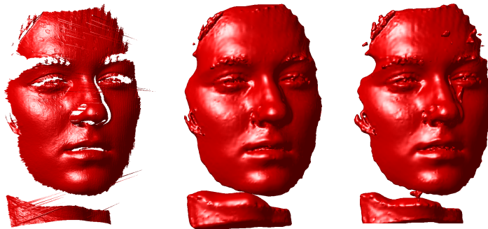
Figure 3.7: The outlier noise in the left scan was automatically removed with our method using a linear loss function (centre). For the squared loss function (right) even the best parameter set produced some spurious surfaces.
